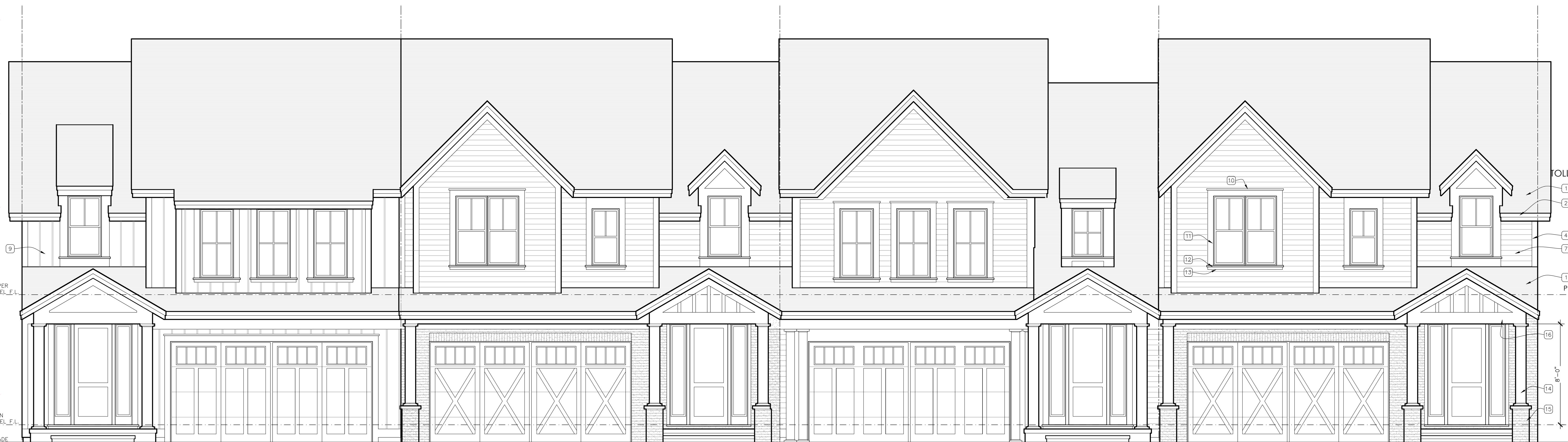
2-STORY CARRIAGE HOUSES - FRONT ELEVATION SCALE: 1/4" = 1'-0"
