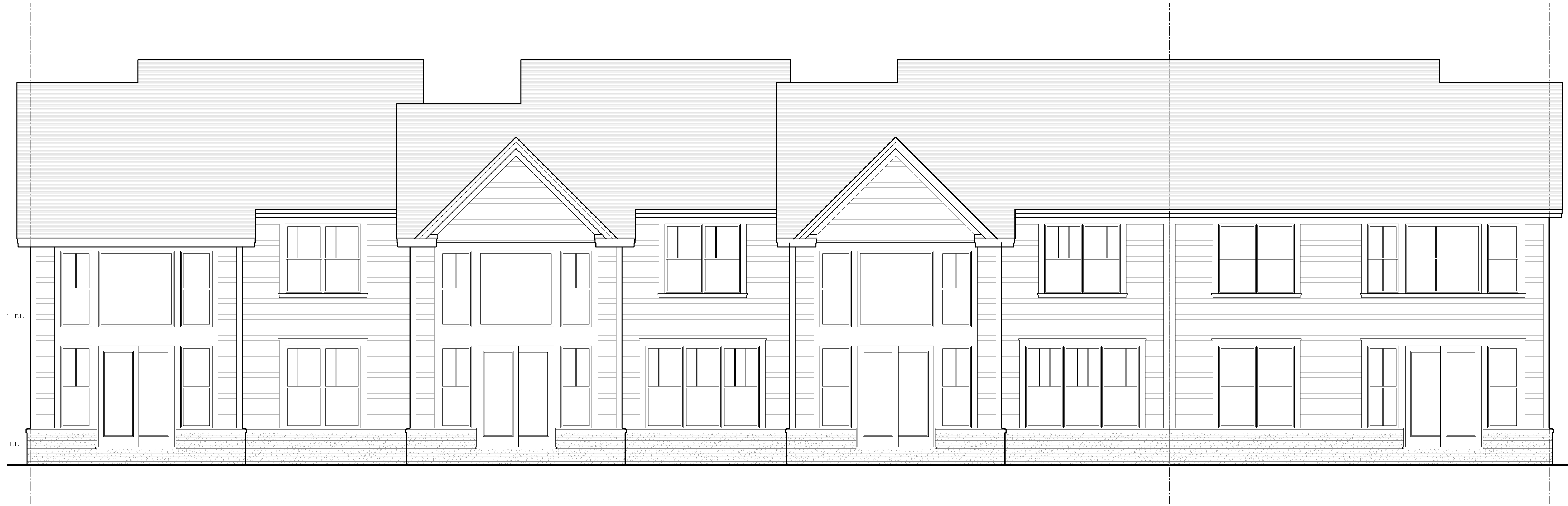
2-STORY CARRIAGE HOUSES - REAR ELEVATION SCALE: 1/4" = 1'-0"
