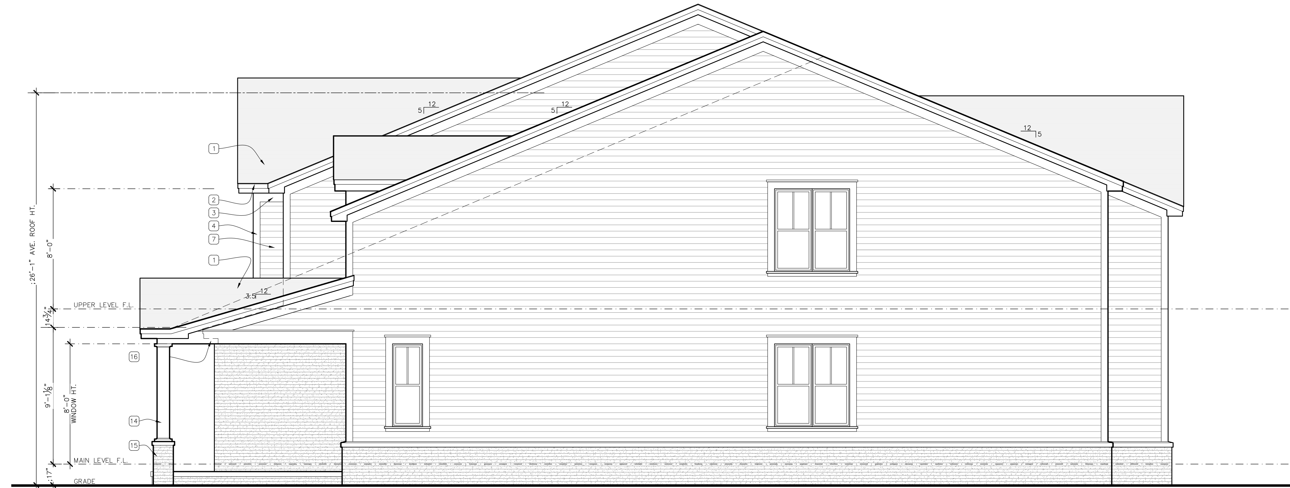
2-STORY CARRIAGE HOUSES - SIDE ELEVATION SCALE: 1/4" = 1'-0"
