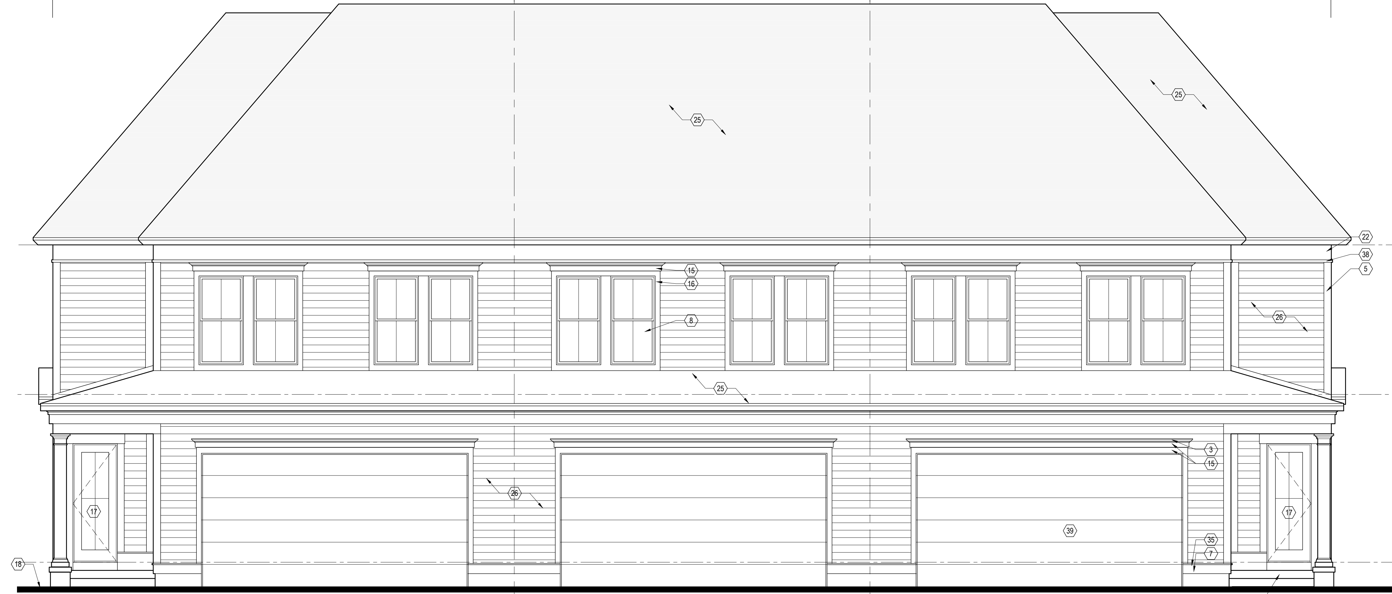
1 EAST ELEVATION A312 1/4" = 1'-0"
