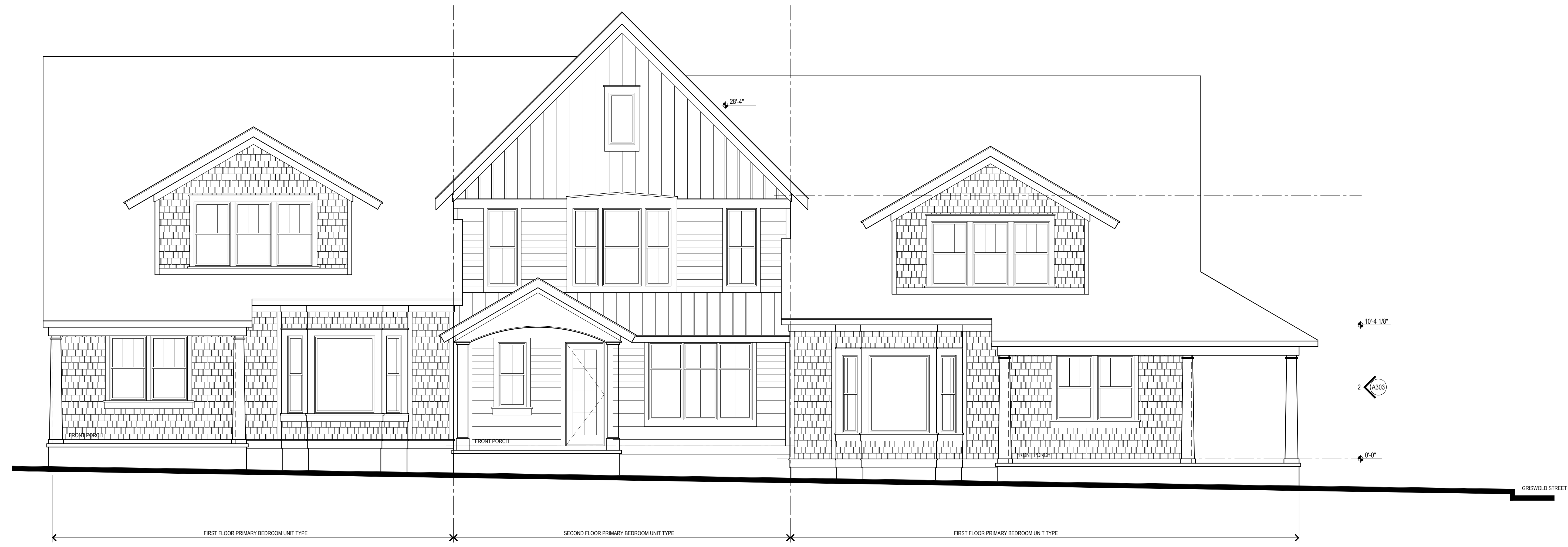
2 SOUTH ELEVATION - BEAL STREET A302 1/4" = 1'-0"
